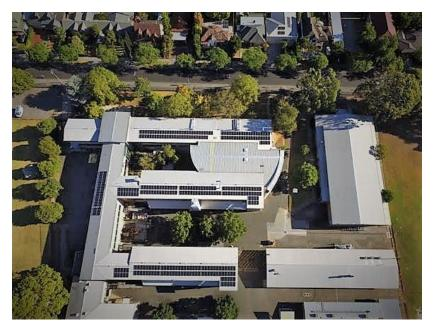
The SolarEdge system is connected to the internet, to allow login via portal on any device to monitor system performance, system status and access detailed output graphs over time. An estimated yearly energy saving of 165.278 MWh and an extended warranty, the system is envisaged to provide ongoing contribution to the school's energy needs for the future and a great benefit to the environment.
